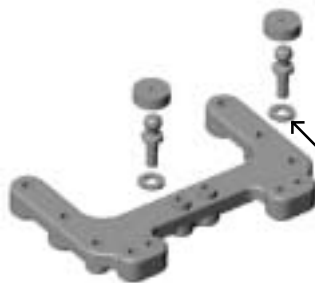
Raise or lower the ball end by adding or subtracting washers here
