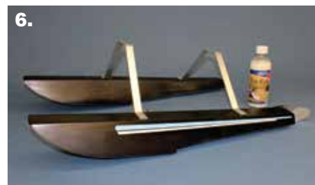
Fig 6. The floats have been painted black, decorated with stick-on plastic trim, ready for mounting.
