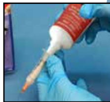
Fig 1. First, a syringe is filled with R/C Modellers Canopy Glue, right out of the tube.
