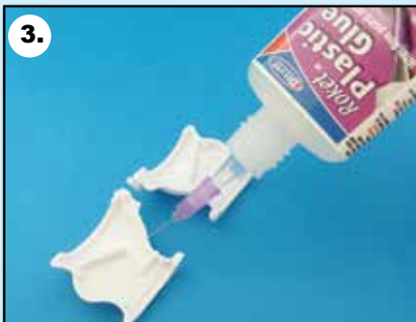
Fig 3. To join the toilet bowl, use Roket Plastic Glue or Plastic Magic 10 Sec Cement . It allows a longer working time & can be spread thinly over both sides of the bowl without evaporation.
