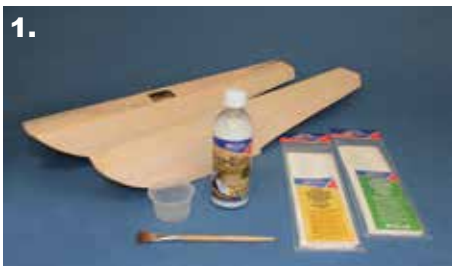
Fig 1. All you will need is a bottle of Eze-Kote, a selection of Deluxe Super Lightweight Glass Laminating Fabric, a small cup & a paintbrush.
