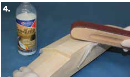
Fig 4. After drying, excess fabric can be effortlessly trimmed away using 320 grit sand paper.
