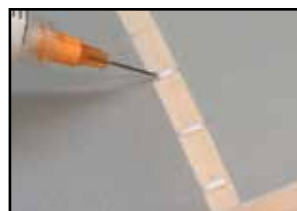
Fig 2. Wing rib stitches are simulated with the smaller syringe tip, carefully running glue lines on predetermined marks across the wing rib caps.
