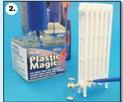
Fig 2. Using Plastic Magic AD77 , assemble the radiator. Identify & join the four centre sections first using the fine point brush for intricate joints.
