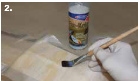
Fig 2. After an initial coat of Eze-Kote has been applied & allowed to dry, a piece of 0.6oz Glass Laminating Fabric is cut & laid on the surfaces.
