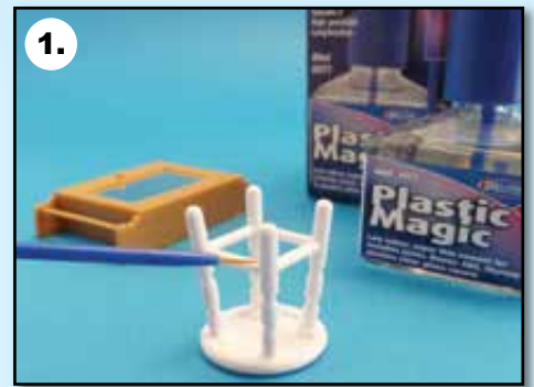
Fig 1. Use Deluxe Materials Plastic Magic to assemble the stool. It is ideal for close fitting joints as it acts quickly. The bathroom cabinet was assembled similarly.
