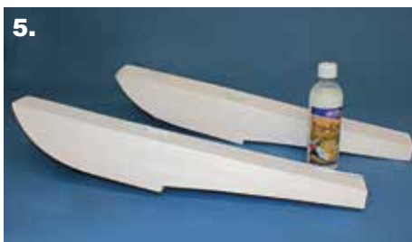
Fig 5. Both floats have been covered, sanded & primed.
