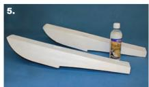
Fig 5. Both floats have been covered, sanded & primed.
