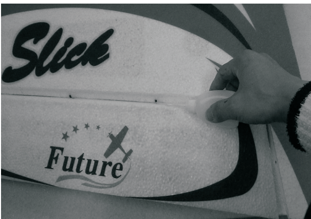
23. Install aileron and stick the hinge with glue. Leave 1mm between the aileron and wing, so that it can be risen and down very flexible
