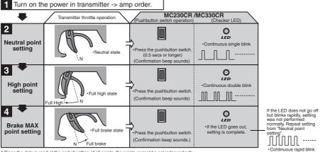
\* Since the data is read at the end of setting of all points, the points cannot be set independently. If the amp power was turned off during setting, the setting points cannot be memorized. (The previous settings are retained.) \* The confirmation heen sounds only when the motor was connected.
