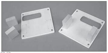
□ □ 1. Trim the covering from the servo arm cutouts in the aileron and flap (if you will have operational flaps) servo hatch covers. Use epoxy to glue the 3/4" x 3/4" x 5/16" [19 x 19 x 8mm] hardwood servo mounting blocks to the inside of the aileron and flap hatch covers. Be sure that the blocks are aligned
