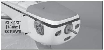
□ 4. Drill 1/16" [1.6mm] holes at the marks you made on the cowl through the cowl mounting blocks. Remove the cowl and thread a #2 x 1/2" [13mm] self-tapping screw into each hole in the cowl mounting blocks and back it out. Apply a couple drops of thin CA to each hole in the blocks. Enlarge the four holes in the cowl with a 3/32" [2.4mm] bit. Install the cowl onto the fuselage using four #2 x 1/2" [13mm] self-tapping screws and four #2 flat washers.
