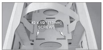
□ 4. Fit the fuel tank tray into the fuselage by inserting the tab at the forward end of the tray into the slot in the firewall. Press the tray down onto the receiving tabs in the fuselage former and cross brace. Drill two 1/16" [1.6mm] holes through the tray and into the hardwood mounting blocks. Secure the tray in place using two #2 x 1/2" [13mm] screws and two #2 flat washers, being sure to harden the screw holes with thin CA.
