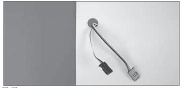
$\Box$  13. Route the servo lead(s) through the hole in the top of the wing panel.
