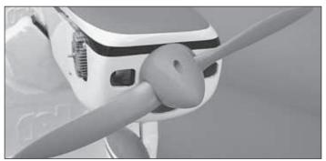
□ 5. If necessary, ream or drill the spinner backplate to fit the crankshaft of your engine (or brushless motor prop adapter). Install the backplate onto the crankshaft followed by the propeller. Install the prop washer and prop nut. Depending on the size propeller you are using, you may need to enlarge the propeller blade cutouts in the spinner cone. When a good fit is achieved, use the screws included with the spinner to install the spinner cone onto the backplate.
