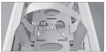
□ 5. Fit the fuel tank tray into the fuselage by inserting the tab at the forward end of the tray into the slot in the firewall. Press the tray down onto the receiving tabs in the fuselage former and cross brace. Drill two 1/16" [1.6mm] holes through the tray and into the hardwood mounting blocks. Secure the tray in place using two #2 x 1/2" [13mm] screws and two #2 flat washers, being sure to harden the screw holes with thin CA.
