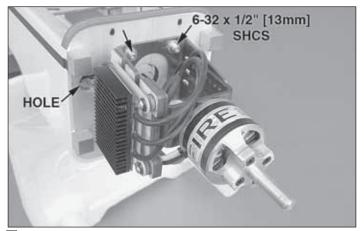
□ 6. Drill a hole in the firewall for the battery lead from the ESC and the receiver lead. Attach the motor mount to the firewall using four 6-32 x 1/2" [13mm] SHCS, four #6 flat washers, four #6 lock washers, and threadlocking compound. Connect the motor leads on the ESC to the motor. Be sure that the leads will not interfere with the rotation of the motor.
