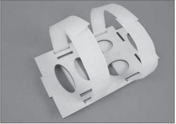
□ 4. Make two 12" [305mm] long hook and loop straps from the included hook and loop material by overlapping the mating ends of each side by approximately 2" [51mm]. Insert the straps into the slots in the plywood **fuel tank tray** as
