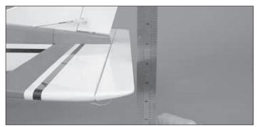
Use a Great Planes AccuThrow<sup>™</sup> (or a ruler) to accurately measure and set the control throw of each control surface as indicated in the chart that follows. If your radio does not have dual rates, we recommend setting the throws at the low rate setting.
