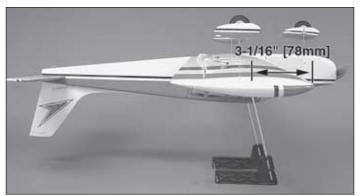
□ 2. With the wing attached to the fuselage, all parts of the model installed (ready to fly) and an empty fuel tank, place the model upside-down on a Great Planes C.G. Machine, or lift it upside-down at the balance point you marked.
