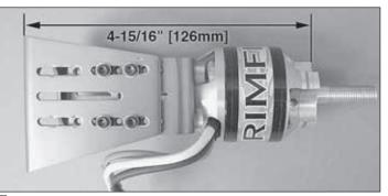
□ 1. Attach the out-runner motor to the brushless motor mount using the included 3 x 8mm machine screws and threadlocking compound. If you haven't done so yet, install the prop adapter to the motor case with the hardware included with the motor and threadlocking compound. Loosen the screws that hold the two motor mount halves together and set the distance from the back side of the mount to the front of the prop adapter to be 4-15/16" [126mm]. Retighten the screws using threadlocking compound.
