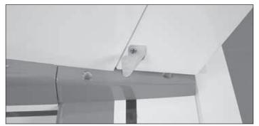
□ 4. Install a control horn onto the left side of the rudder in the same manner.
