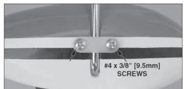
□ 3. Place a landing gear strap over each gear leg and mark the locations for the screw holes. Drill 3/32" [2.4mm] holes at your marks, being sure not to drill into the wheels. Install a strap onto each pant using two #4 x 3/8" [9.5mm] selftapping screws. Reinforce the holes with thin CA.
