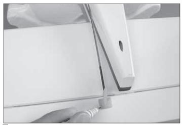
□ 2. Temporarily insert a 36" [914mm] pushrod into the elevator outer pushrod tube that exits the right side of the fuselage. Use the position of the pushrod to mark the location for the elevator control horn onto the underside of the elevator.
