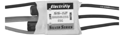
ElectriFly Silver Series 12 (SS-12) ESC (GPMM1810) for 12A maximum constant current draw.
