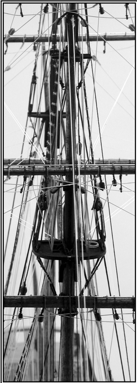
FIG. H-11 GAFF VANGS, BOOM TOPPING LIFTS & SHEET
