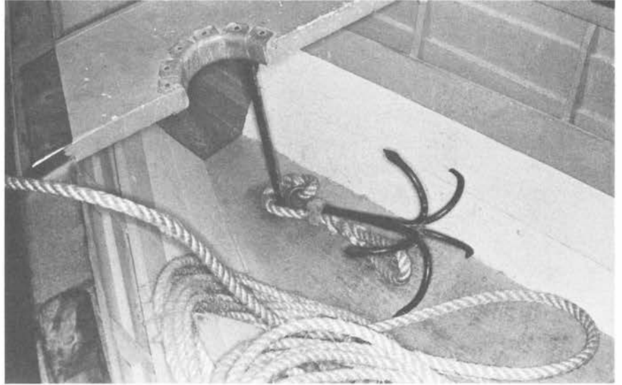
Figure 2-12. The bow of the Lagoda model's port bow boat, showing the thigh board and leather lining of the clumsy cleat. The five-prong grapnel is unusual, as surviving examples in New Bedford Whaling Museum have only four prongs.
