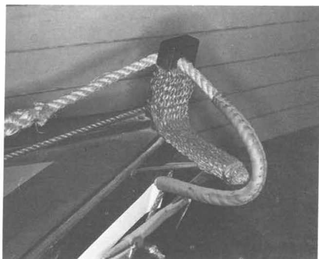
Figure 2-10 (left). The steering oar brace on the Lagoda model's port spare boat (stowed upside down on the boat skids).
