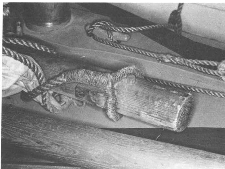
Figure 3-120. The head of the mast of Lagoda's waist boat, showing the served eye of the shrouds, the shoulder cleat (the shroud has been shifted, but the cleats should support it at the splices), and the wooden peg to prevent the shrouds from slipping off.
