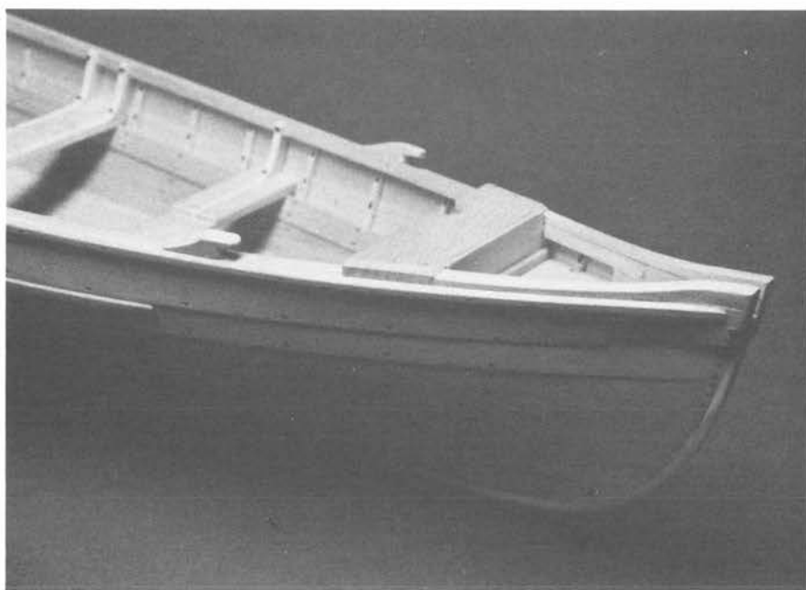
Figure 3-79. The bow, showing the addition of the preventer cleats, bow chocks, and the box. Note the addition of rivets to the forward ends of the cheek pieces where they join the stem post.
