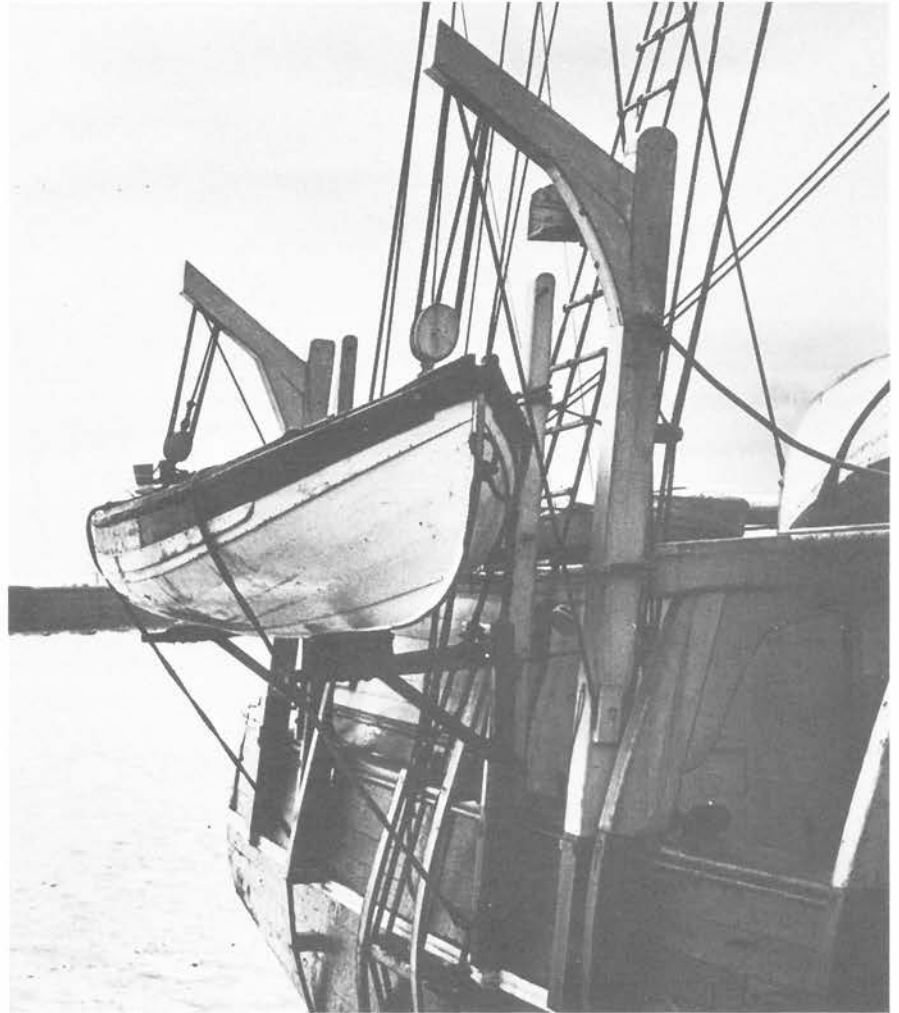
Figure 1-2. The New Bedford whaleboat in its final development was 29-30 feet in length, depending on the type of whaling intended, 6-6½ feet in beam, and planked in a combination lapstrake and batten-seam style. Photograph by Albert Cook Church. Old Dartmouth Historical Society
