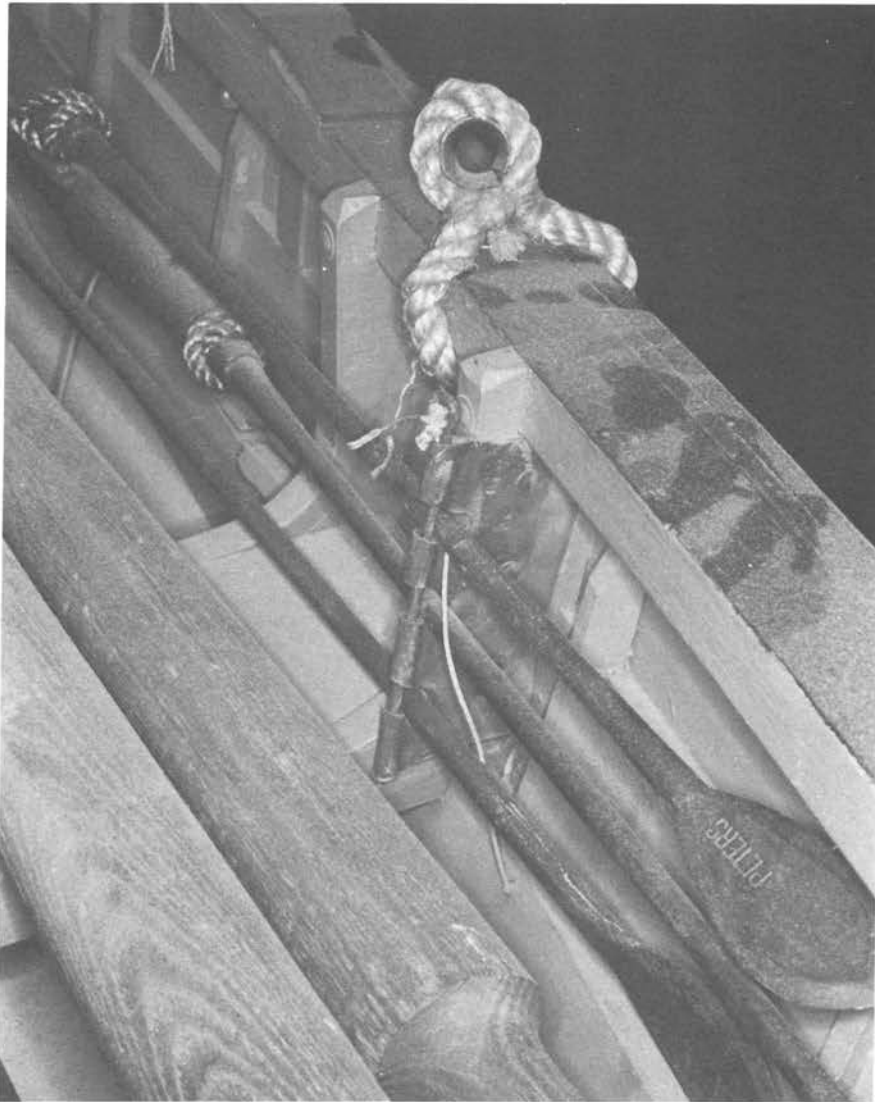
Figure 2-15. The Lagoda model's waist boat, port side, with its lances stowed in the rack at the mast thwart. The stamp on the lance head is that of Ambrose and Charles Peters, who ran the last blacksmith shop in New Bedford to specialize in whalecraft.
