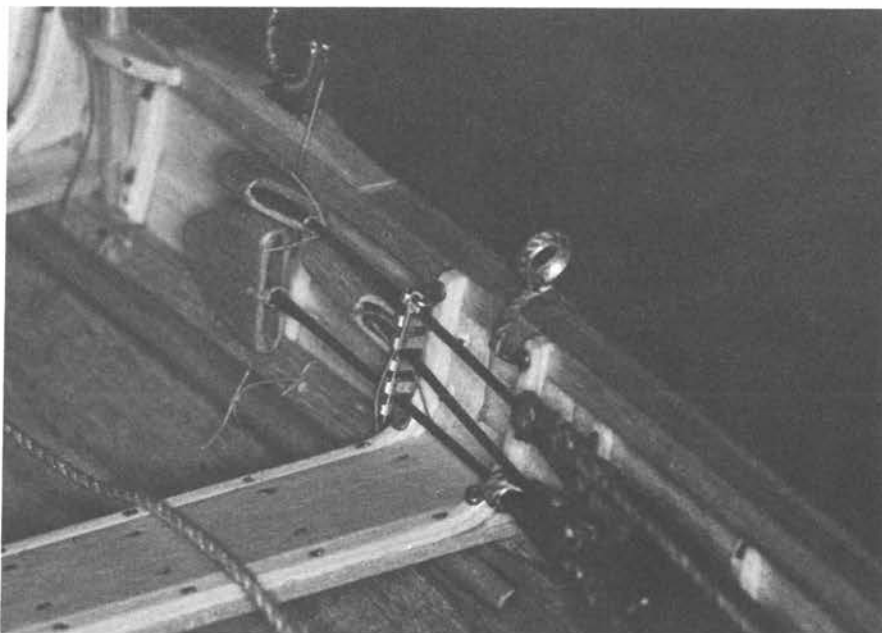
Figure 3-130 (left). Inboard view, starboard side, showing three harpoons in the rack (there is space for two more). The harpoon heads are fitted with sheaths (above). The racks are formed from .010" copper or brass sheet. Begin by doubling a piece \frac{1}{2} " \times 1" around a short length of #28 gauge wire (A) and crimping the fold in a vise or pliers (B). Slots are sawn or filed (D) and the rack is trimmed and drilled (E). The racks are fastened to the filler pieces of the thwart knees with copper nails (F). Note that the lance rack has only three slots (E).
