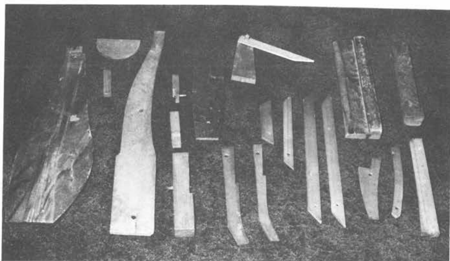
Figure 4-11. Patterns and marking gauges made and used by Joshua H. Delano when he built the whaleboats for the Lagoda model. The patterns for the rudder, mast hinge block, lion's tongue, and quarter "stiffeners" are readily identifiable. The straight pieces with sharp ends are probably patterns for the beams which supported the bow and stern sheets. Other pieces are depth and marking gauges and a beveling gauge. Photograph by the author
