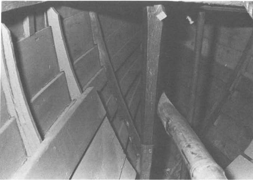
Figure 1-8. The stern of a 30-foot whaleboat built for the Arctic fishery, ca. 1895, looking under the cuddy. The upper three seam battens are visible at left-center; above them are the laps of the sheer and gunwale strakes. Note the notches in the frames and damage to the one at far left. Between it and the next frame aft can be seen a backing block on the gunwale strake where two planks have been scarfed and fastened. Photograph by the author
