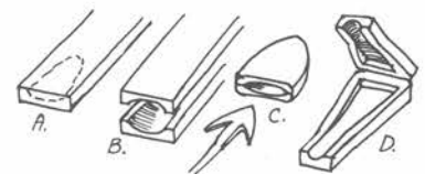
Figure 3-131. Fabrication of sheaths for whalecraft. Steps A-C show the fabrication of a sheath for a double-flued harpoon head; see plans, Sheet 3 for details of other types of lance and harpoon sheaths. The boat spade sheath (D) opens like a clam shell and has a leather hinge (not visible).
