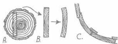
Figure 4-10. Cross-section of a whaleboat's planking, showing growth rings with their heartwood sides facing outboard. A, a plank as cut from the log; B, the tendency of cedar to "cup" during the drying process; C, utilization of this characteristic in planking and ceiling the shell.
