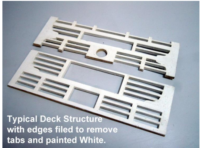
Deck Structure sections laser cut in carrier sheets with joint details also laser cut into surface of wood.
