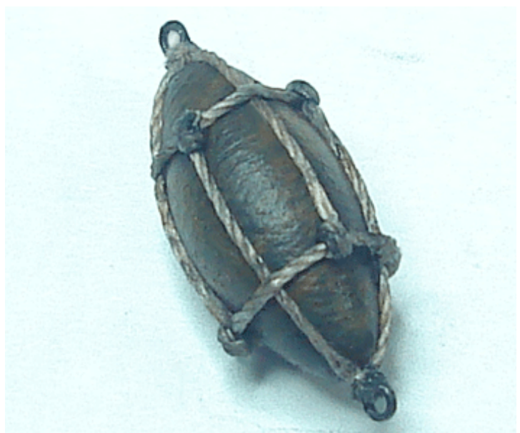
Completed buoy. Note how the harness legs go under the other harness as the work their way down to be lashed to the base of the eyebolt.
