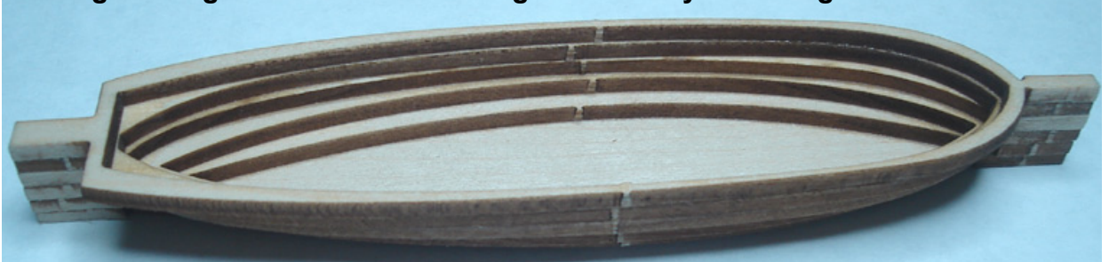
Lifts glued together with the tabs aligned. The Syren's longboat has five lifts.
