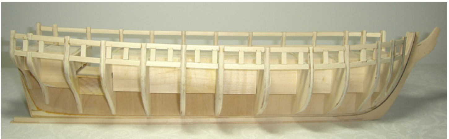
All of the green frames are glued into place. These frames define the sides of the gunports.
