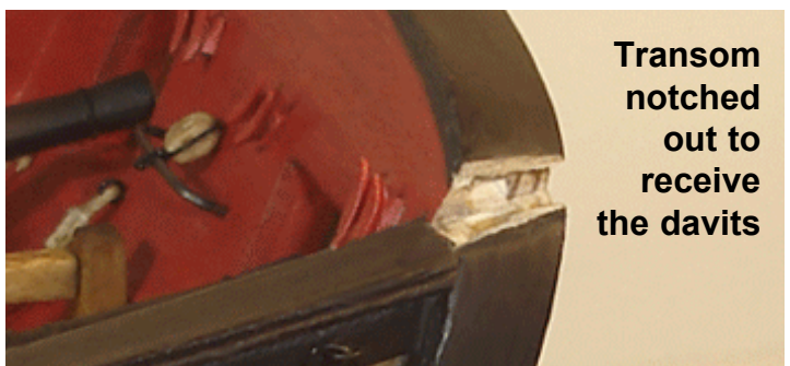
Stern davits in place, The cleats have not been glued into position yet.
