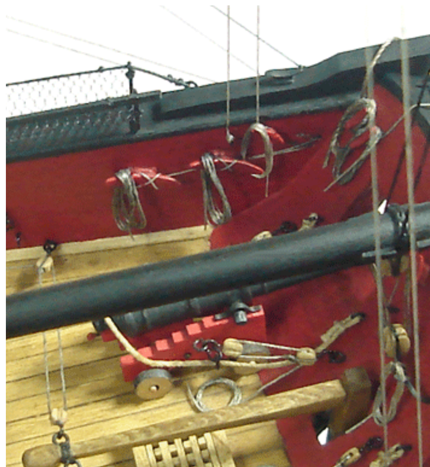
These two photos show the inboard portions of the main course sheets and braces (below) and the fore sheet (above). It is best if you add these soon before getting to much rigging done. It will be easier to complete them with less rigging to get in the way. Not shown is the main tack which is handled in the same way.
