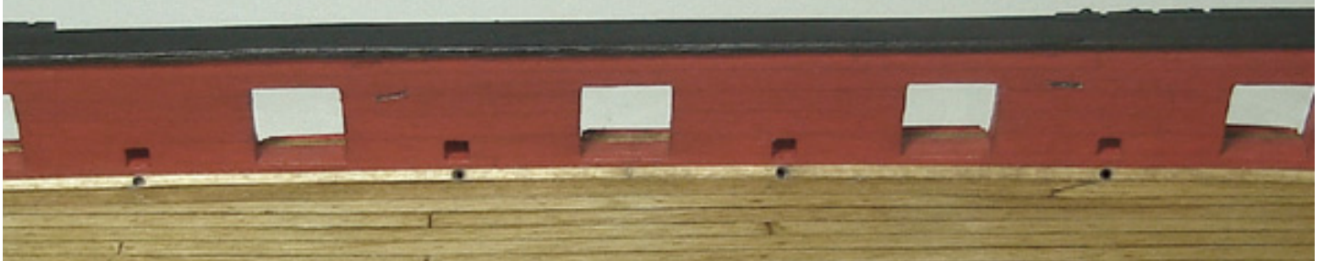
Inboard look at the scuppers and sheaves
