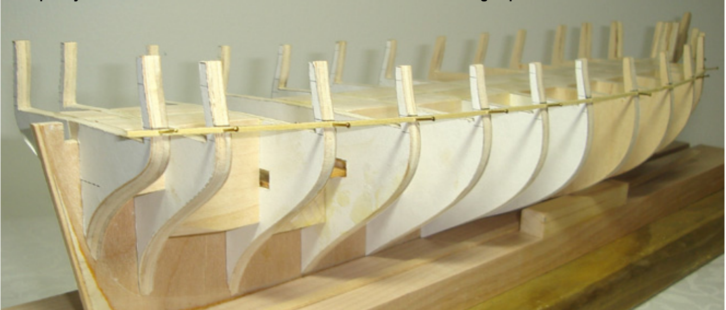
Temporary batten fastened to the hull to establish the smooth run of the gun port sill.
