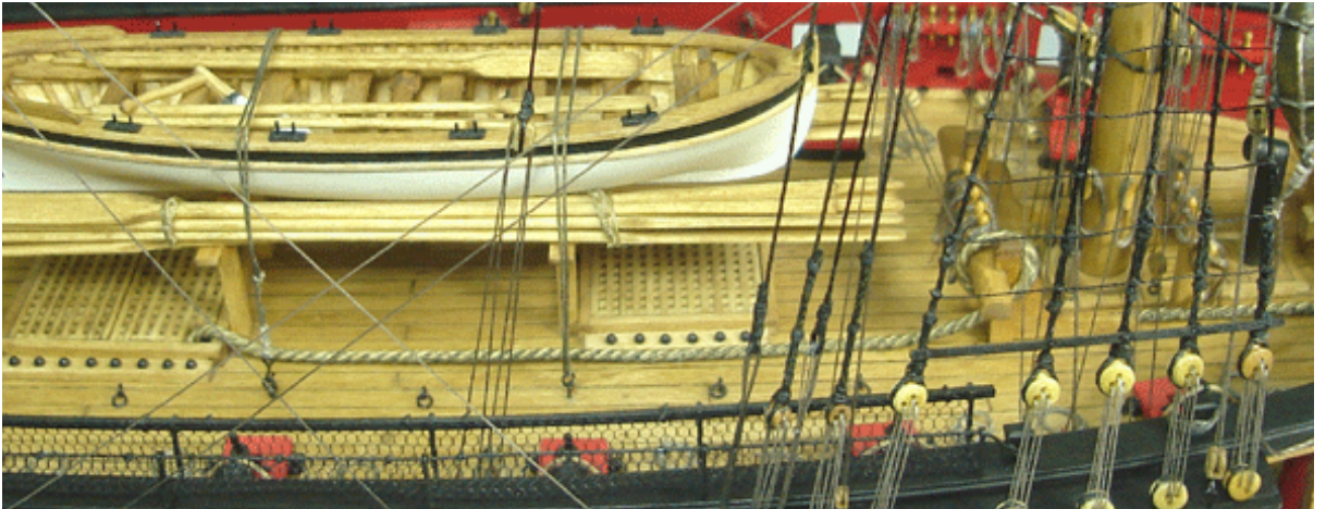
Anchor cable taken around the riding bits and led into the holes in the hatch gratings.
