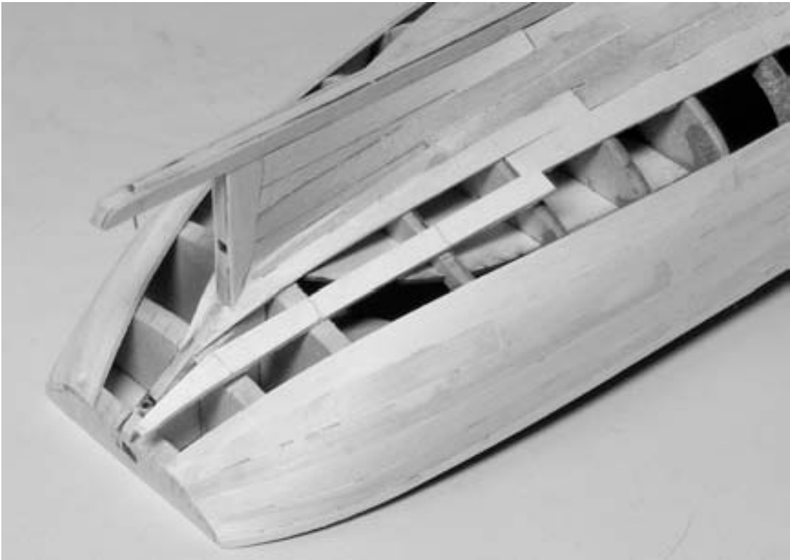
Photo 7: The shape of planks at the stern
