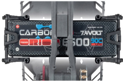
LONG BATTERY INSTALLATION
