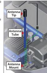
tighten the screw just until the antenna tube is securely in place. Do not over tighten. Do not bend or kink the antenna wire! See the sidebar for more information. Do not shorten the antenna tube.
