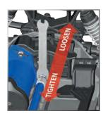
Place the model on a high-traction surface, such as carpet. Adjust the slipper so that you can hear it slip for approximately two feet from a standing, full throttle start. (Learn more about adjusting the slipper clutch in the sidebar.)
