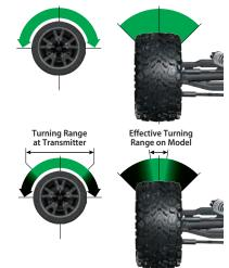
sensitivity may be helpful when driving on low-traction surfaces, when driving at high speed, or on tracks that favor sweeping turns where gentle steering inputs are required. The ranges are exaggerated for illustrative purposes.
