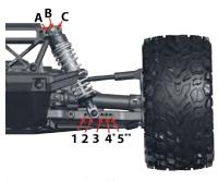
settings help reduce body roll (increased roll stiffness), dive during braking, and squat during acceleration.
