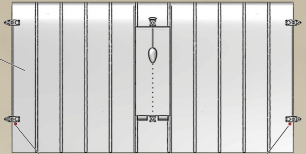
Upper centre section & 25 gallon gravity petrol tank
