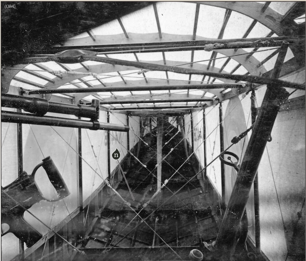
The inside of the rear hull from Felixstowe F.3 (not F.2a) N4408. Note the 2 side mounted Lewis guns and the upper gun dangling upside down from its mounting. The rear hull sides and top coamings of N4408 are obviously CDL while the bottom and washboards have received a coat of protective black bituminous tar based paint. Unlike the F.2a, the tapering top coaming of the F.3 extended all the way to the leading edge of the fin. It appears that much of the internal bracing cables have been painted, possibly in bright colours to make them more visible and/or to resist corrosion. Note the substantial padding applied to the 'X' bracing cables beneath the aft cockpit hatch.
