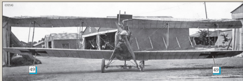
This front view of DFW C.V 799/17 allows us to see the highly translucent nature of the wings which would indicate that the camouflage colours used on the upper surfaces were tinted varnishes which were not opaque. Note the damage to the leading edges of the top wings, damaged port wheel and broken propeller blade serving witness to the circumstances of its capture.
