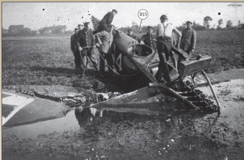
The crash and recovery of DFW C.V (LVG) 'white 4' from Schusta 26 allows us to see several interesting details. Note the style of the exhaust which is almost exclusively found on LVG built DFW C.V, the small support brackets from the cabane to the radiator and the square white fields behind the wing and fuselage eisernkreuz. These white fields were eliminated in a directive sent in October 1916 which would indicate that this aircraft is from a production order placed that month with LVG for 50 DFW C.V (numbers 7650/16 to 7699/16).
