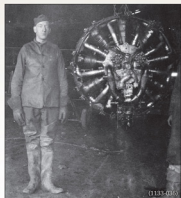
This photo of an American serviceman allows us to see the rear of a Salmson 9z engine which is hanging from a block and tackle.
