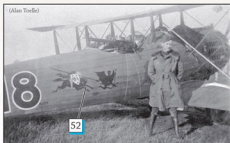
Salmson 2-A2 '18' showing some repaired 'battle damage' above the unit insignia and patched fuselage fabric covering a previous installation of the external generator partially hidden by Phil Henderson in this photo.
